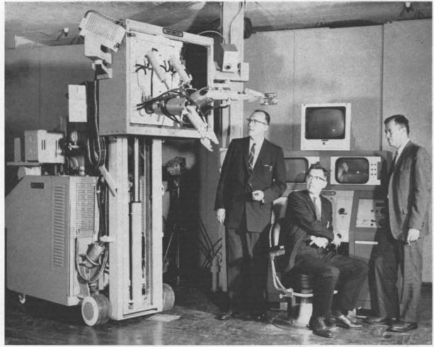
"SANDY MOBOT," a remote mobile handler designed for use in Sandia's SERF reactor facility, will be operating in front of the "Sphere of Science" during the New Mexico State Fair. Shown
